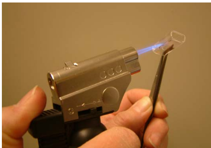
Figure 4-18. Cleaning the glass cell with a micro torch.
