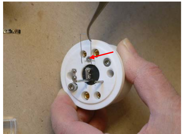
Loosen the screw holding the spring for the glass cell, and remove it carefully.
